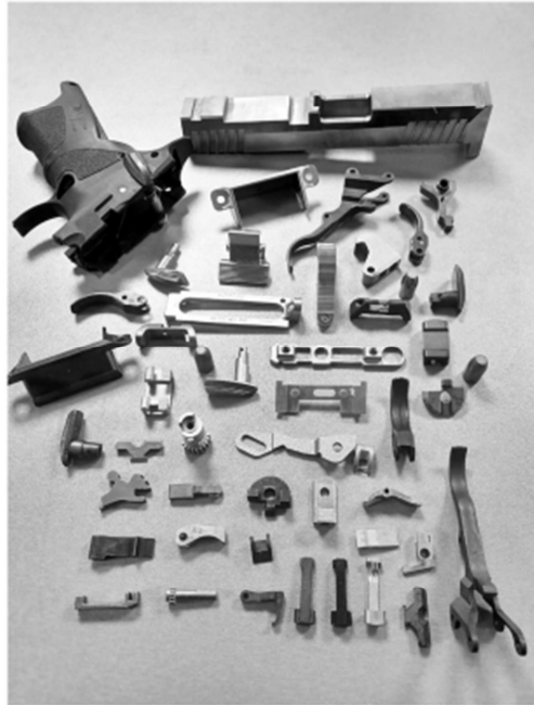
Fig. 10 A selection of MIM and PM parts, including at the top, a large MIM firearms component (Courtesy Gevorkyan)
