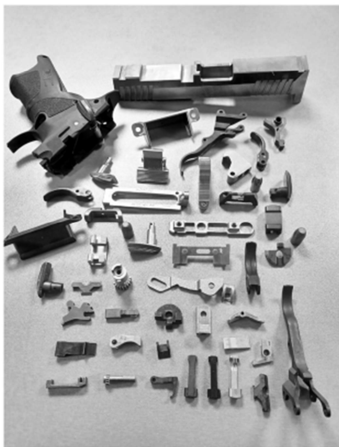
Fig. 10 A selection of MIM and PM parts, including at the top, a large MIM firearms component (Courtesy Gevorkyan)
