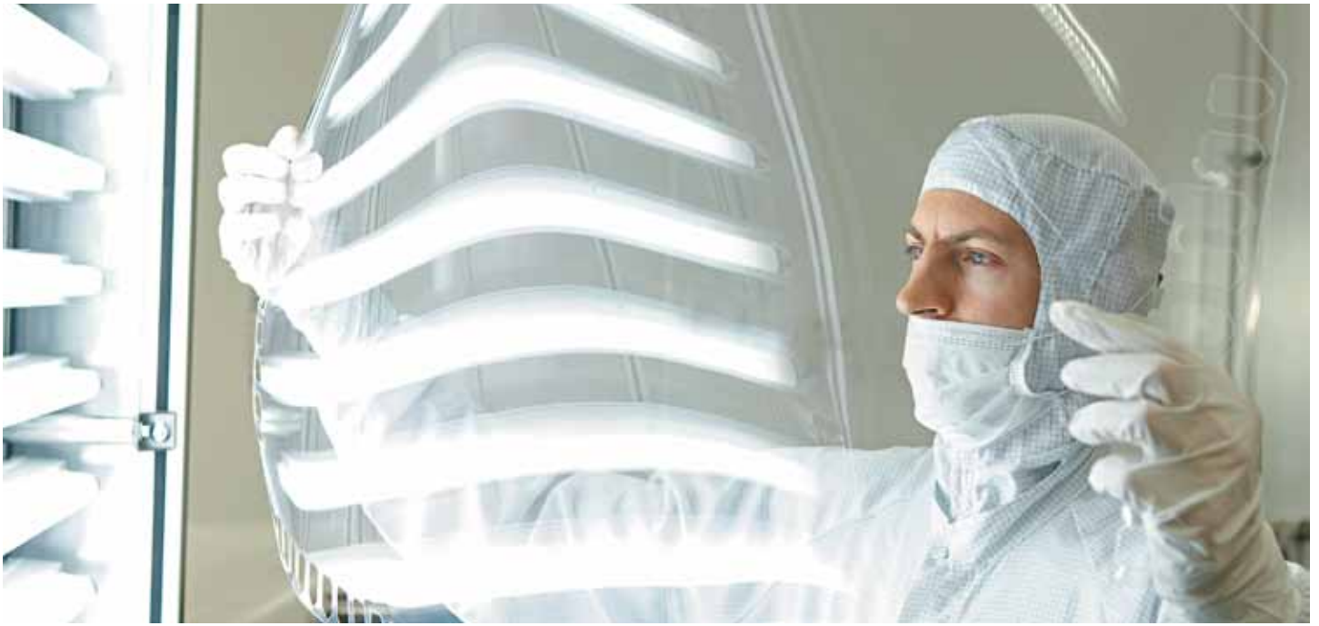
Webasto Glas ProTec® is thin and light: In the clean room process, a highly tear-resistant PET film is applied to thin sheets of glass.
