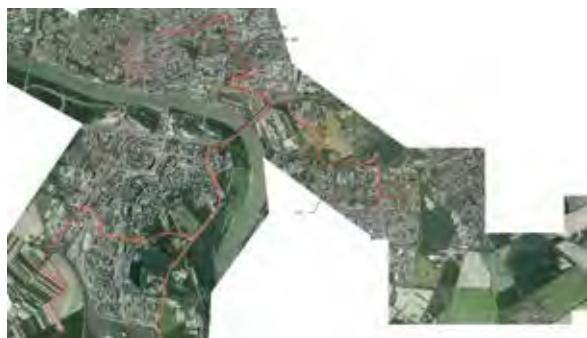
Bratislava's optical cables in the RIS database also underwent a complete renovation. The problem was outdated data due to the fact that most of the optical cables were not outlined. Nevertheless, thanks to archive data we managed to create a coherent picture of optical cables in Bratislava. In the next period, we plan to outline more cables and the data on cables will be also updated in RIS.
